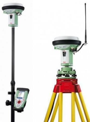
Figura 4.1 - GPS GS-15 Leica®.
